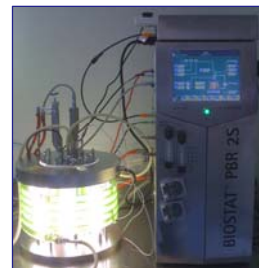
Fig.5 Sartorius® photobioreactor used to investigate growth and H 2 production kinetics
